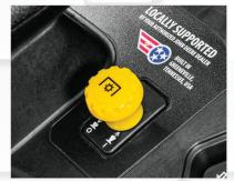
Electronic mower deck engagements increase efficiency with the pull of a button.
