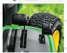
Two-pedal hydrostatic transmissions make maneuverability smooth & simple.
